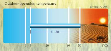
Toshiba MiNi-SMMS 7 is designed to perform cooling operation up to 50°C, this guarantees high reliability of our product even at high ambient temperature.
